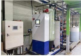
**NiCycle** recovers nickel ions from most post-electrolytic nickel-plating rinses and returns a high purity-, high concentration nickel sulphate or nickel chloride solution that can be reused in most electrolytic plating solutions.
